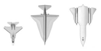
Figure 4. Aircraft Size Comparison: An F-15, the RASCALAircraft, and the SR-71
